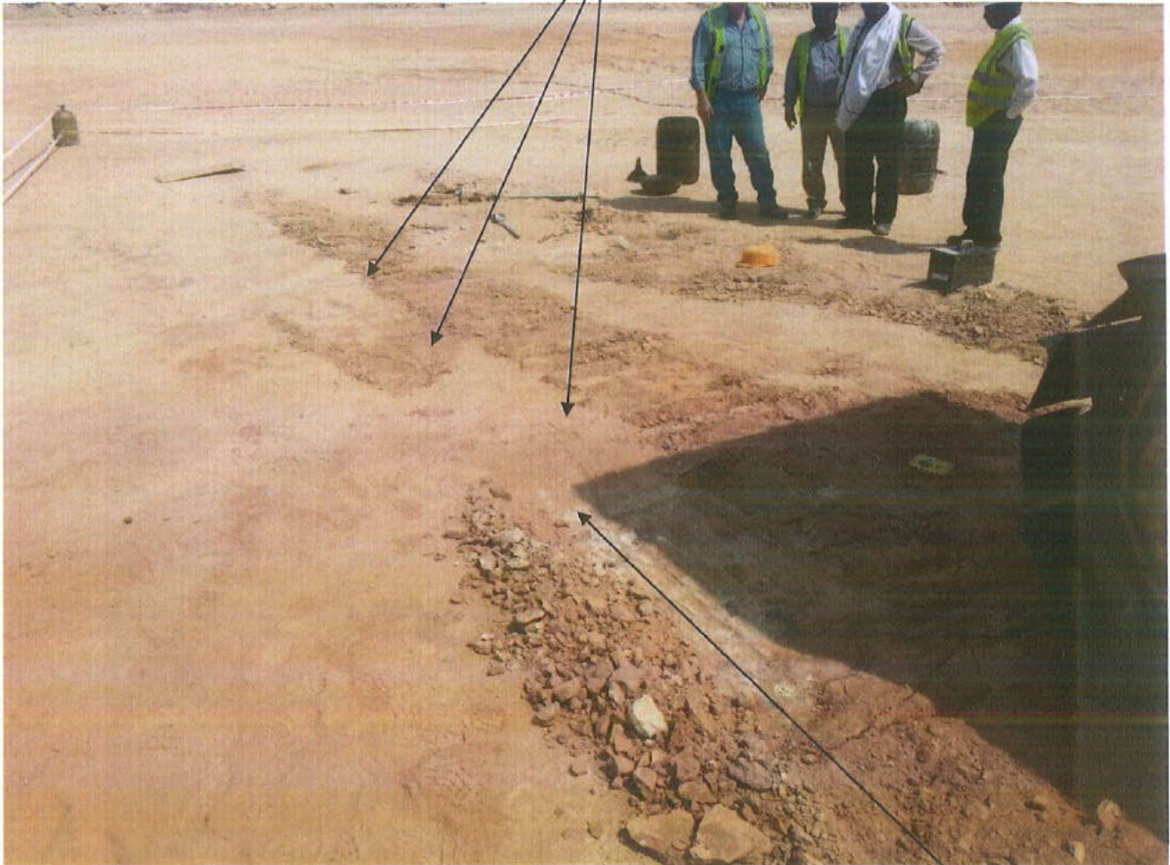
Blade marks increased in depth at this position indicating blade was lowered by (b)(6)
