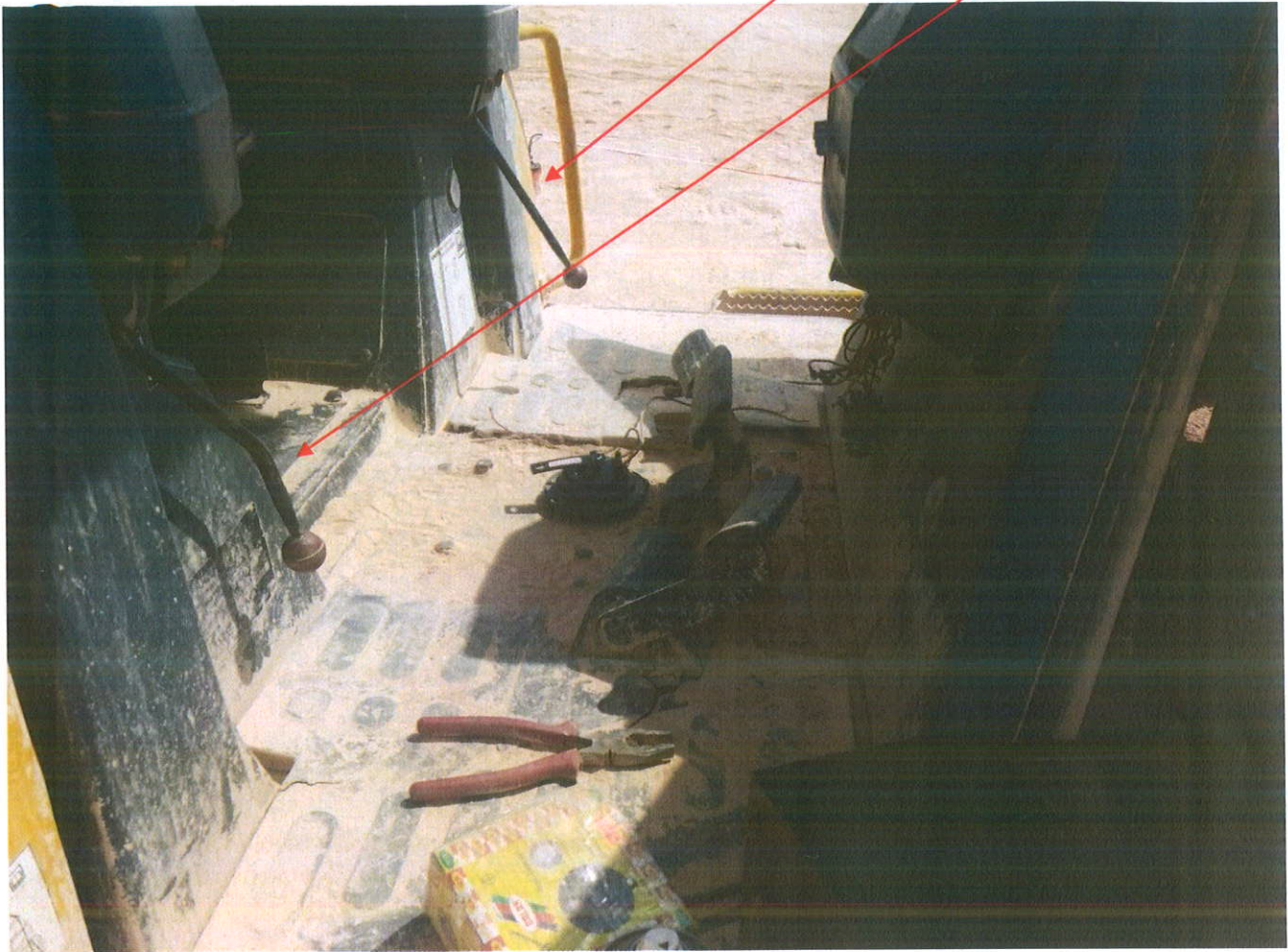
Photo 4 showing replacement Horn and tools used by Electrician, Park Brake and Blade Control Levers in locked position
